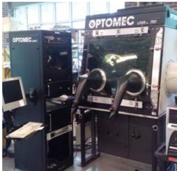
Figure 2.8 LENS machine used to fabricate Ti-6Al-4V thin wall.
