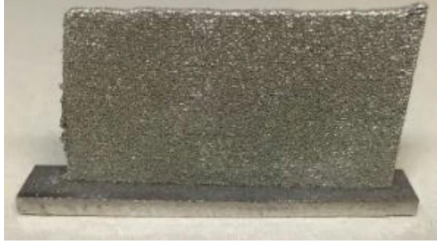
Figure 2.9 Fabricated Ti-6Al-4V thin wall using LENS machine.
